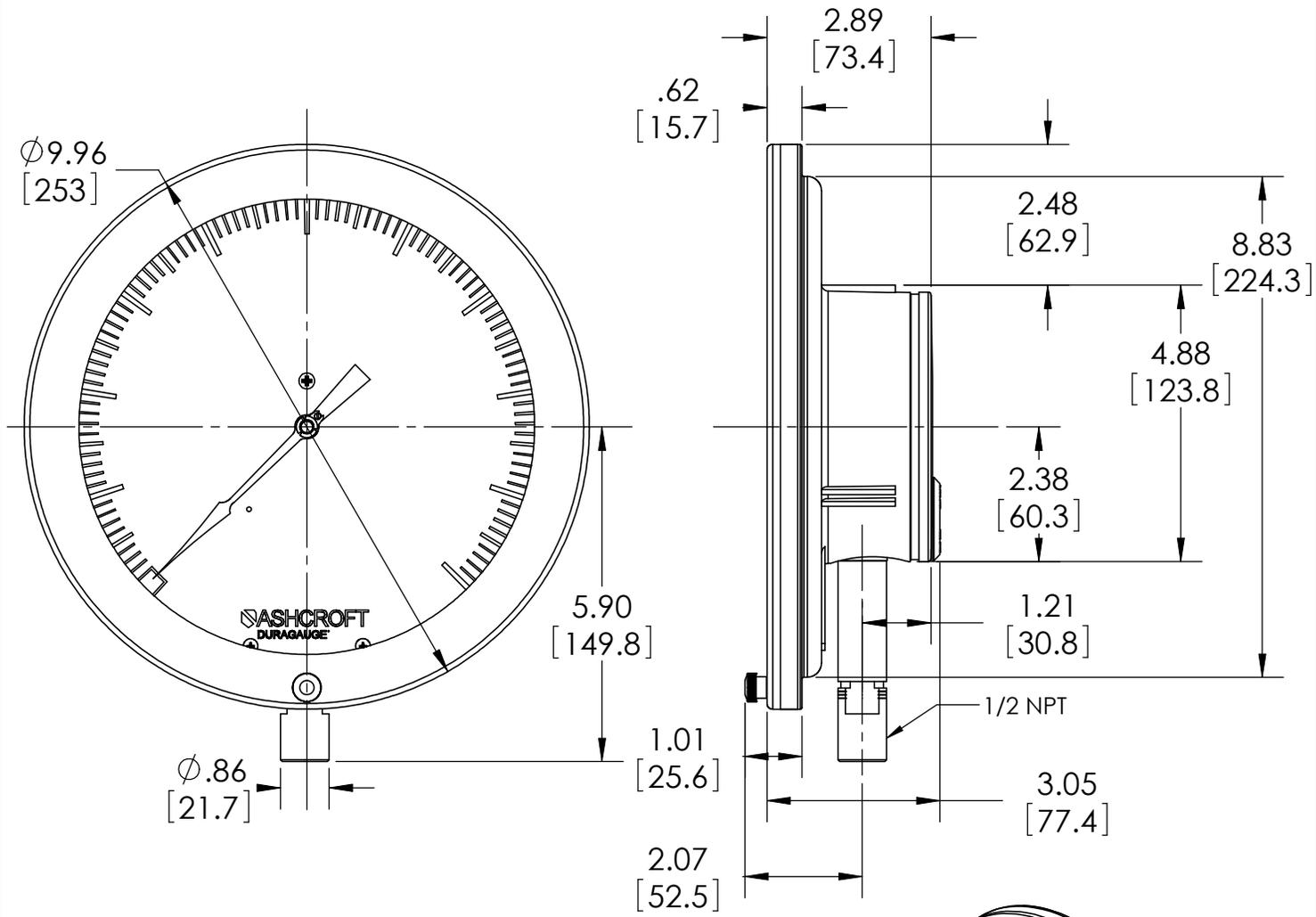
Note: 3 Mounting studs threaded equally spaced on a 9.625" [244] Bolt Circle.
